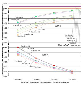
The height of the towers depends on the distance of the towers and therefore on the mirror area concentrating the solar radiation onto each receivers and therefore on the power the receivers are designed for. Estimations of the peak power, of the needed tower height and the number of towers depending on the receiver design and the given ground area will be presented as well.
