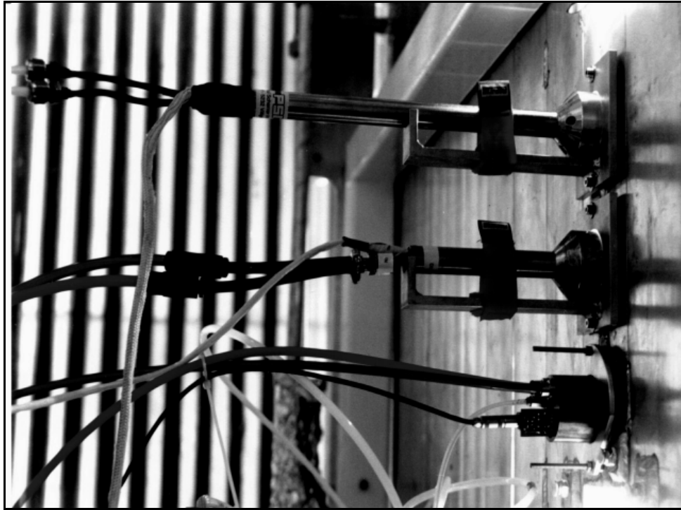
Fig. 1: Detailed look on three fluxmeters mounted in a cooled panel (backside) in the focal plane of the 1MW solar furnace in Odeillo, France.
